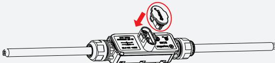
*Note: Under the circumstance that need to remove the inverter AC cable from 3P-AC bus connector, please use the 3P-AC connector unlock tool and insert the tool into the side of AC port to remove.*
