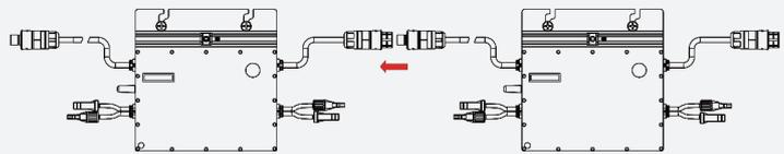
*\*Note: The length of AC cable on microinverter is roughly 2.06 m, if the distance between two microinverters is more than the AC cable, please use an AC extension cable between two microinverters (as shown in the picture on the right).*
