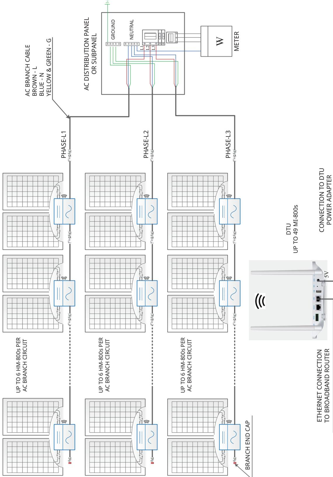
WIRING DIAGRAM – 120 VAC/208 VAC THREE-PHASE:
