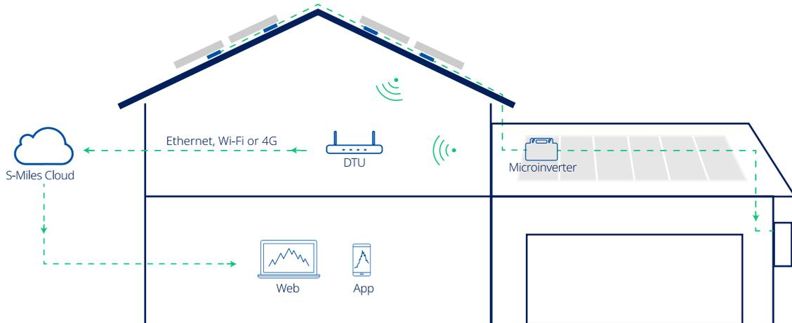
The complete Hoymiles PV microinverter system is composed of PV microinverter, Hoymiles gateway DTU and Hoymiles monitoring system S-Miles Cloud.
