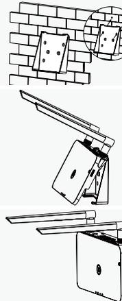
Option 2: Place the DTU on table. Please make sure the antennas are vertical to the table.
