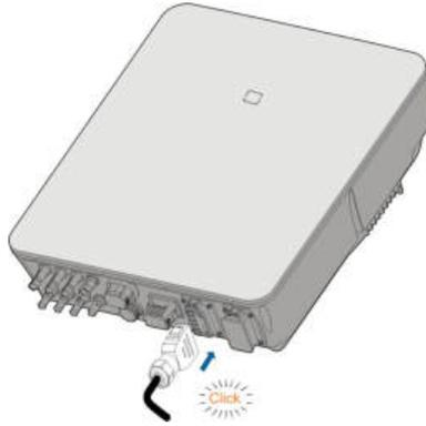
step 4 Pull all the lines outward to check whether they are firmly installed.
