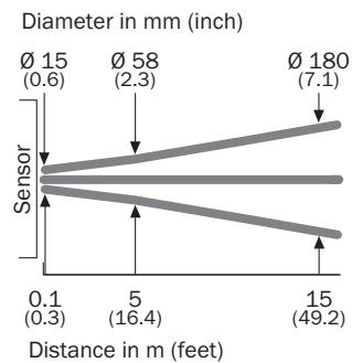
Sensing range diagram GL10, Logistik, DC, GL10G, DC
