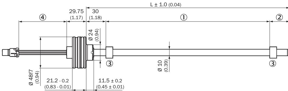
Dimensional drawing M12 connector type L/ flange - radial seal
