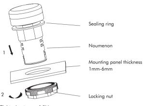
Tightening torque 1.8N·m
