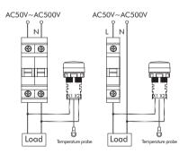
ND 3-22T,ND 3-22T/S wiring diagram
