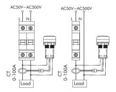
ND3-22A, ND3-22A/S, ND3-22AV/S, ND3-22AV,ND3-22AVHz/S wiring diagram
