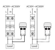
ND3-22V, ND3-22V/S wiring diagram
