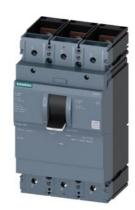
switch disconnector 3VA1 IEC frame 400 3-pole SD100, In=400A without overload protection w/o short-circuit protection nut keeper kit
