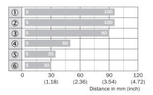
$\blacksquare$  Max. sensing range  $S_n$ , flush or non-flush installation, non-magnetizable material
