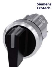
Illuminable selector switch, 22 mm, round, metal shiny, black, Selector switch short, 3 switch positions I>O<II, momentary contact type, actuating angle 2x45°, 10:30h/12h/13:30h
