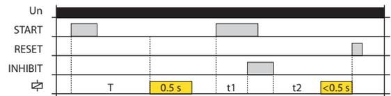
When the supply voltage is applied, the relay is open. When the START control contact is closed, starts the time delay T. After the end of the timing relay switches for the fixed time (0.5 sec).
