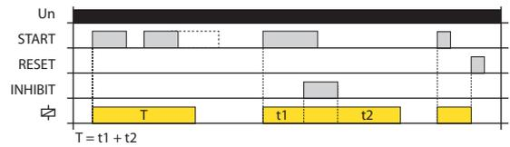
When the supply voltage is applied, the relay is open. When the START control contact is closed, the relay energizes and starts the delay time T. After the end of the timing relay is switched off. The closing of the START control contact during timing is ignored.
