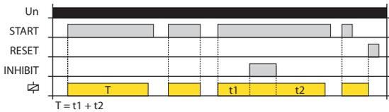
When the supply voltage is applied, the relay is open. When the control contact START is closed, the relay closes and the time delay T begins. If the START control contact is open during timing, the time interval is immediately terminated and the relay opens.
