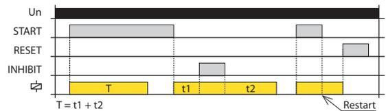
When the supply voltage is applied, the relay is open. When the START control contact is closed, the relay energizes and starts the delay time T. After the end of the timing relay is switched off. By opening the control contact start relay again closes and starts the delay time T. After the end of the timing relay is switched off.
