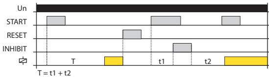
When the supply voltage is applied, the relay is open. If the control contact START is closed, the time delay T starts. The closing of the START control contact during timing is ignored.
