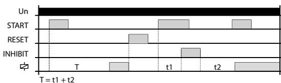
When the supply voltage is applied, the relay is open. If the control contact START is closed, the time delay T starts. The closing of the START control contact during timing is ignored.
