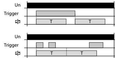
When the supply voltage is applied, the relay is open. When the control contact is closed, the relay closes and the time delay T begins. When the control contact is opened, the relay closes and the time delay T begins. If the control contact is open during timing, the relay remains closed for 2T. When the timing is complete, the relay opens. Any other change of control contact status during timing is ignored.
