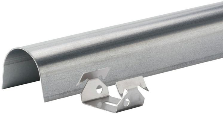
The innovative cable protection system from ABB makes installing protection for cables faster, easier and providing a sleeker outlook. The system includes metal quick clamp and straight 1200 mm long covers with a corrosion resistant Magnelis® coating. Available in four different sizes (16, 22, 28 and 34 mm).
