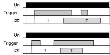
When the supply voltage is applied, the relay is open. If control contact is closed, time delay T starts. When the control contact is opened, a new time delay T begins. If the control contact is open during timing, the relay closes at the end of the timing and opens the relay after the new time delay. Any other change of control contact status during timing is ignored.
