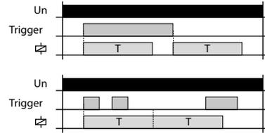
When the supply voltage is applied, the relay is open. When the control contact is closed, the relay closes and the time delay T begins. When the control contact is opened, the relay closes and the time delay T begins. If the control contact is open during timing, the relay remains closed for 2T. When the timing is complete, the relay opens. Any other change of control contact status during timing is ignored.
