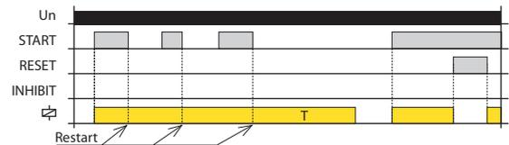
If the START control contact is open during timing, a restart occurs - the relay remains closed and a new time delay T begins. When the timing is complete, the relay opens.
