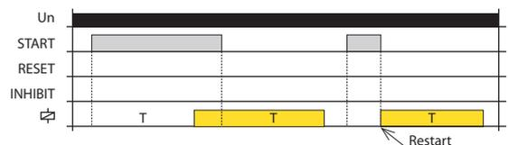
If the START control contact is open during timing, a restart occurs - the relay closes and a new time delay T begins. When the timing is complete, the relay opens.
