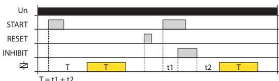
When the supply voltage is applied, the relay is open. When the START control contact is closed, starts the time delay T. After the end of the timing relay closes and again runs delay time T. After the end of the timing relay opens and the sequence is repeated until the supply voltage is disconnected.
