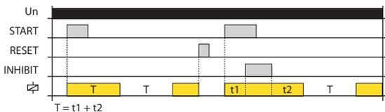
When the supply voltage is applied, the relay is open. When the START control contact is closed, the relay energizes and starts the delay time T. After the end of the timing relay opens and again runs delay time T. Upon completion timing again switches, and the sequence is repeated until the supply voltage is disconnected.
