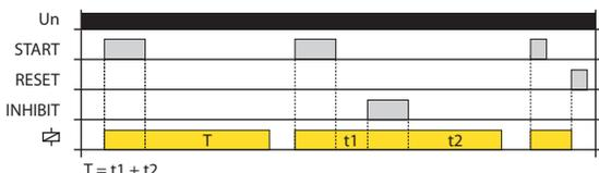
When the supply voltage is applied, the relay is open. If the control contact START is closed, the relay closes. After tripping Contact Start starts the delay time T. After the end of the timing relay is switched off.
