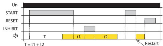
When the supply voltage is applied, the relay is open. When the START control contact is closed, starts the time delay T. After the end of the timing relay switches. Opening the control contact START starts a new time delay T. When the timing is complete, the relay opens.
