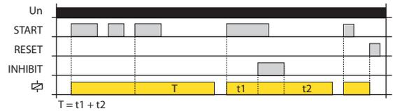
When the supply voltage is applied, the relay is open. When the START control contact is closed, the relay energizes and starts the delay time T. After the end of the timing relay is switched off. Closing control contact START during timing triggers a new time delay T - the relay closing time is thus increased.
