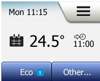
Eco Function reduces the energy spent on unnecessary heating if you leave the room/house during a scheduled heating event. When the Eco Function is enabled, the thermostat enters an energy-saving state, in which the lowest setback temperature in the event schedule is used as the temperature setpoint. At the next scheduled event change, the thermostat returns to normal Scheduled Operation.
