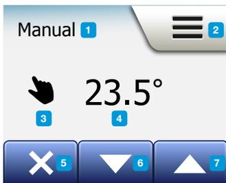
Manual allows you to override Scheduled Operation and maintain a specified temperature around the clock.
