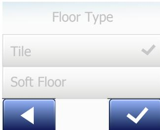
Whenever you change a parameter setting, you must tap the “Accept” button for the thermostat to acknowledge the change. “Accept” is shown on the screen as “√”.
